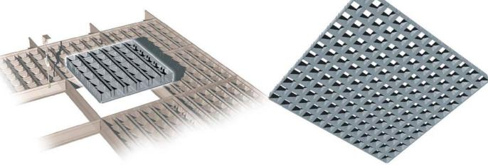
The U-profiles, orthogonally fitted, form modular panels complete with L perimetral profile for the support and the integration in the modular structure constituted by T profiles of 15 mm base. This system allows the use of different typology of panels but with the same module.
